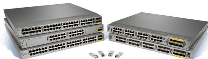
Table 1 summarizes the Cisco Nexus 2000 Series product line. Fabric extenders work in conjunction with a parent Cisco Nexus 5000 or 7000 Series Switch. Cisco Nexus 2000 Series Fabric Extenders can be mixed and matched with a parent switch to provide a variety of connectivity options.
